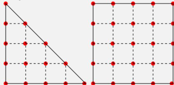
template meta program over reference elements to construct lagrange points
